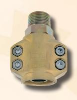
up to +120°C and up to PN 18 bar operating pressure. Female threaded fittings two-piece, rotatable, union nut flat sealing with internal thread sealing ring Frenzelit Novatec Special. Screws for clamping shells DIN 912 - 12.9 (Dacro 500 A coated).
